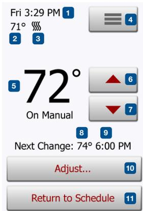
*Note: The temperature set manually on the home screen is a temporary setting. The manual override setting will be automatically canceled at the beginning of the next event in the Scheduled Operation.*
