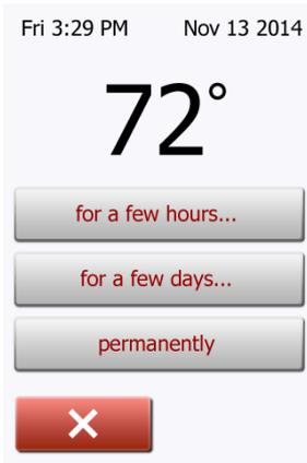
Allows you to maintain the displayed target temperature/setpoint or a Manual Override for longer than just to the next event change or for a specific time period. You can use the “**Adjust...**” options to specify the length of time the displayed target temperature/setpoint should last. When the set time period has elapsed, the thermostat will automatically revert to Scheduled Operation.
