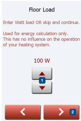
Floor load is used to calculate the energy consumed by the floor heating system. This setting has no effect on floor heating operation.
