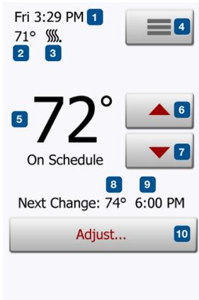
The system will operate in Scheduled Operation unless you choose to override the scheduled events with Manual Operation. During Scheduled Operation, the temperature is controlled automatically according to the programmed heating schedule – see “**Heating Schedule**”.
